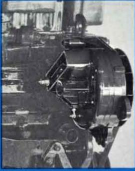
40 amp. alternator is shown here replacing the standard 14 amp. generator. Mounts close to the block.
